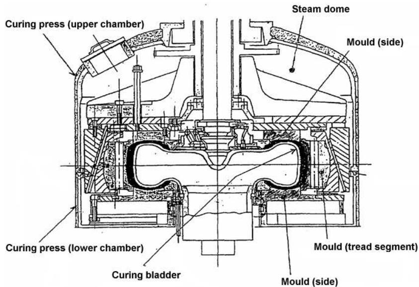
**Fig. 3.** Curing press sketch: this is a vertical section of a steam-dome curing press, highlighting mould, bladder and other components.
